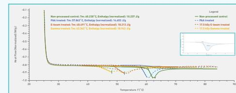
Figure 4: Representative DSC thermograms of different processing groups compared to non-processed control (n=1 per group). Decreased stability of matrix components (denaturation) was indicated by decreasing onset temperatures (Tm). Matrix alteration via crosslinking may be indicated by increasing enthalpy (J/g) values<sup>3</sup>. Widening of transition step curves are evident in both E-beam and Gamma treated samples, also indicating matrix structural changes<sup>3</sup>.
